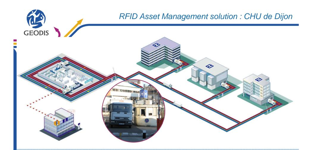
Solution developped to track and trace in the 15 sites of the Dijon CHU, 500 clean and dirty laundry closets via internet with RFID technology.
