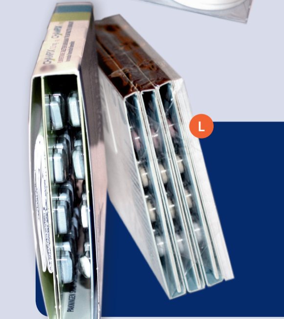
Picture K and L The robot's measuring light will not be able to measure the dimensions due to open or transparent surfaces.
